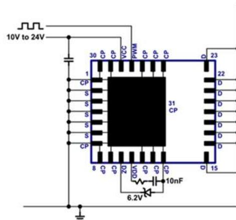
Fig. 18. Start-up circuit
