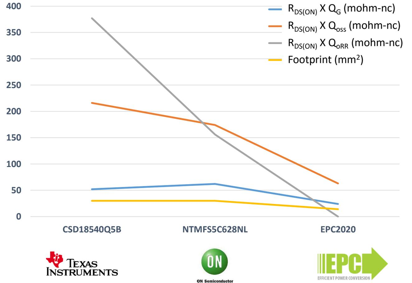
Note: Taken from datasheet typicals at 4.5/5V gate drive and capacitance curves
