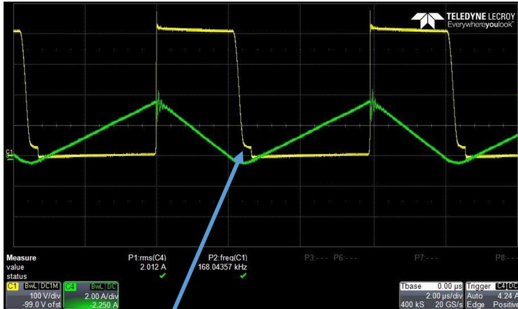
120V<sub>AC</sub>, Si CP partial hard-switching (~200kHz)
