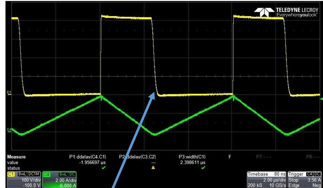
120V<sub>AC</sub>, GaN clean ZVS waveforms (~200kHz)
